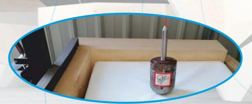
In order to continuously improve the quality of our products, we have developed a special machine to test the strength of our mats by dropping heavy weight from diffrent heights
